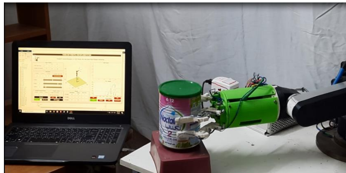
Figure 6: An example of grasping an object to collecting the training data
