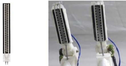
Figure 2: The striped force sensor resistor (FSR type SF10-60)
