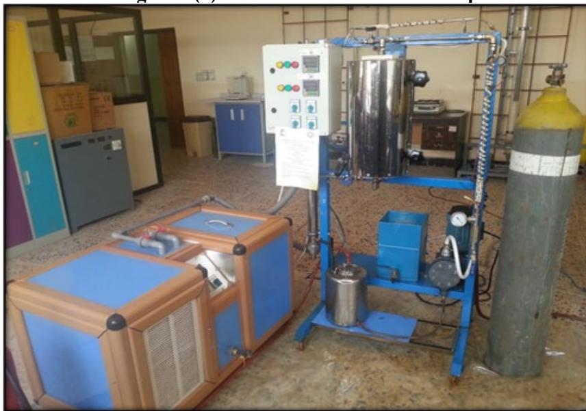
Figure 2(b): Experimental setup of fixed bed reactor.
