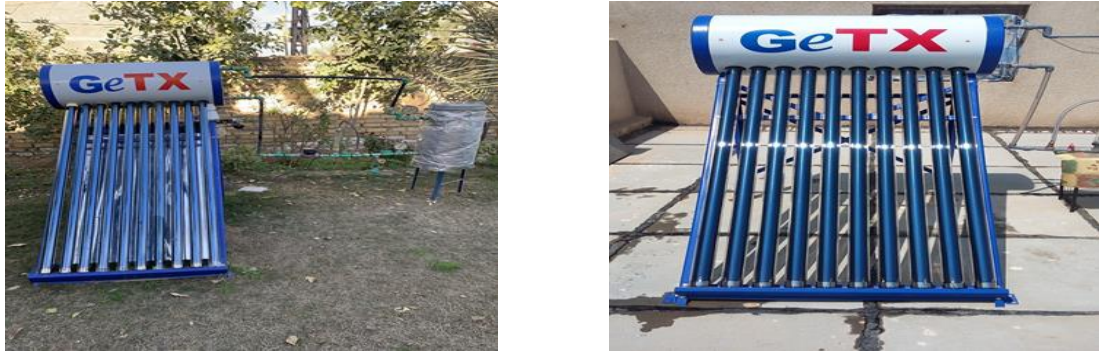
Figure 6: Solar collector with /without reflected curtain
