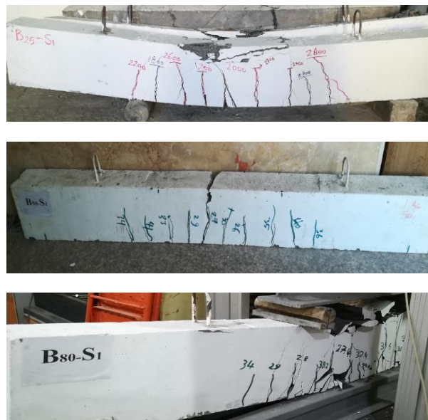
Figure 7: Cracks pattern of beams (25-S1.0), (50-S1.0), and (80-S1.0)
