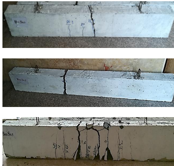
Figure 6: Cracks pattern of beams (25-S0.5), (50-S0.5), and (80-S0.5)
