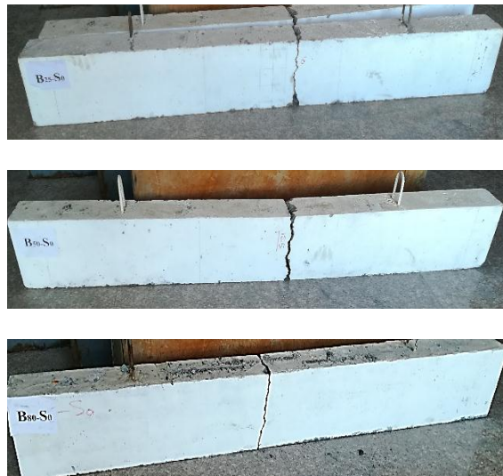
Figure 5: Failure of plain concrete beams
