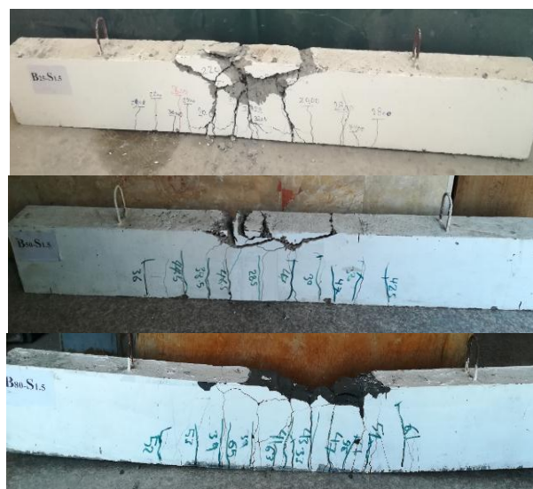
Figure 8: Cracks pattern of beams (25-S1.5), (50-S1.5), and (80-S1.5)
