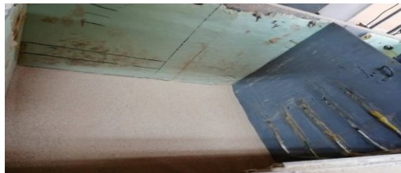
Figure 4: Soil and retaining wall placing in the box.
