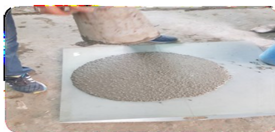
Figure 2: T 500 mm, Slump flow test
