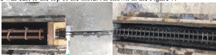
a. The two plates in the side of mold. B. RPC cast in the bottom of the mold.
