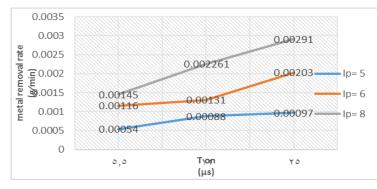
Figure 6: The effect of current and pules of time on MRR for a negative copper electrode
