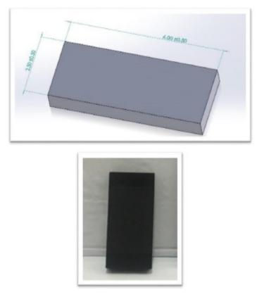
Figure 4: The graphite electrode.
