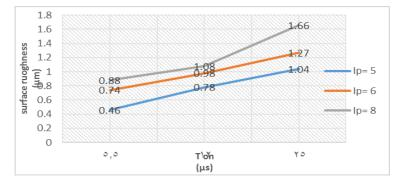
Figure 8: The effect of current and pules of time on SR for a negative copper electrode
