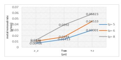
Figure 7: The effect of current and pules of time on MRR for negative graphite electrode
