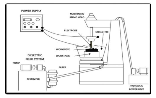
Figure 1: The schematic diagram of the EDM system [6].
