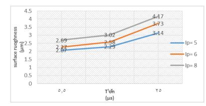
Figure 9: The effect of current and pules of time on SR for negative graphite electrode
