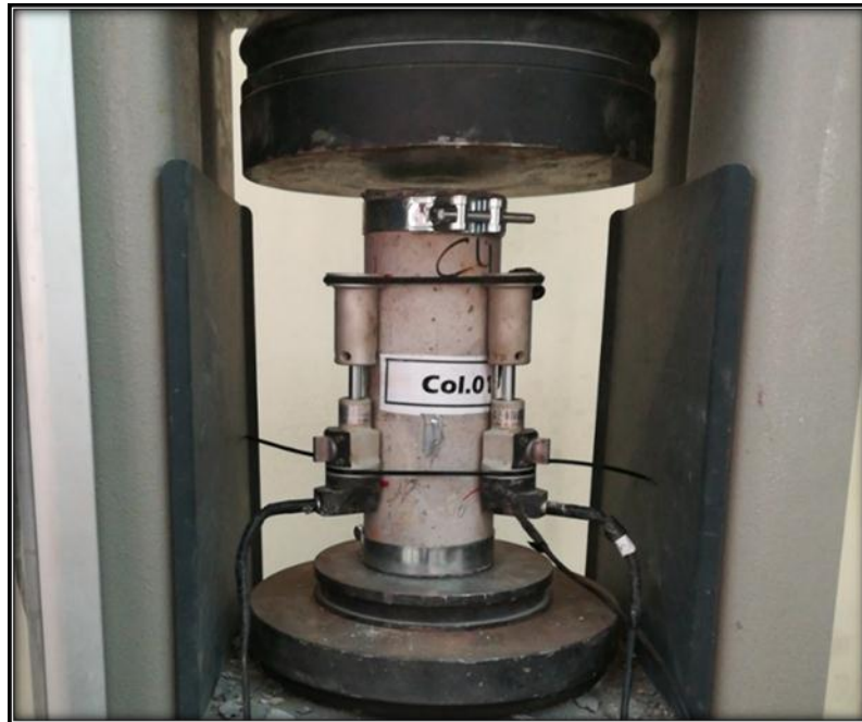
Figure 2: The column specimen under compression load.
