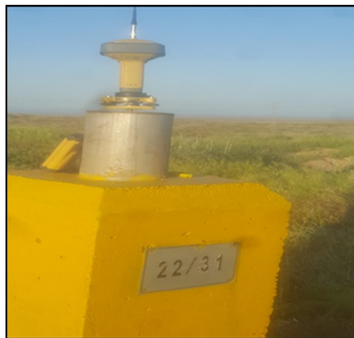
Figure 6: Boundary pillar used as base point for the RTK measurement
