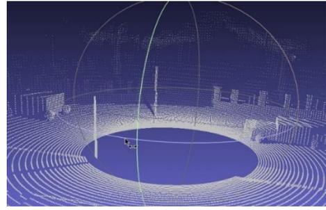
Figure 7: LiDAR output after being processed in MeshLab [28]
