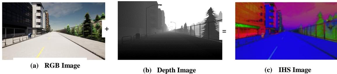
Figure 11: Production of 2.5D image by merge two images RGB & Depth in IHS method
