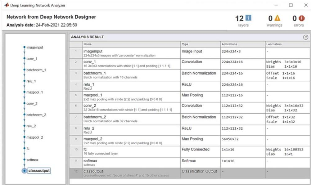
Figure 9: Design of CNN with 12 layers and K-NN classifier
