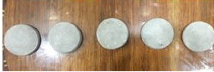
Figure 3: The cement mortars for the hardness and thermal conductivity tests.
