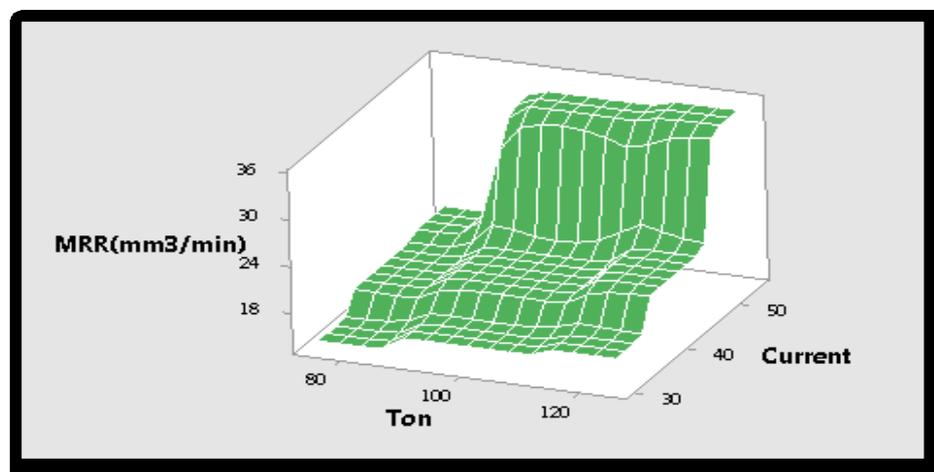
**Figure 5: Plot of Surface for MRR (mm<sup>3</sup>/min) vs Current; Time on**
