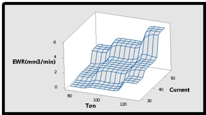
Figure 7: Plot of Surface of Electrode Wear Rate (mm<sup>3</sup>/min) vs Current; Ton
