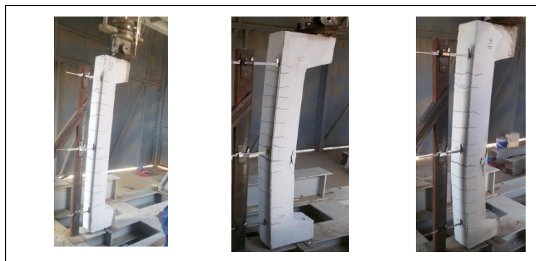
Figure 10: Failure modes for tested columns under eccentric load of 150 mm
