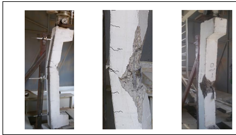
Figure 9: Failure modes for tested columns under eccentric load of 50 mm
