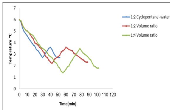
Figure 10: The formation rate CP Clathrate with phenol at 200 ppm and volume ratio 1:2 and 1:4
