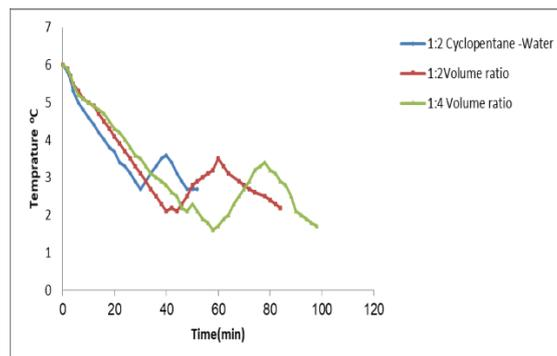
Figure 12: The formation rate CP Clathrate with phenol at 100 ppm and volume ratio 1:2 and 1:4
