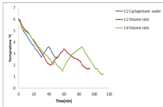
Figure 13: The formation rate CP Clathrate with phenol at 50 ppm and volume ratio 1:2 and 1:4
