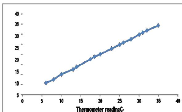
Figure 4: Calibration of the temperature sensor, the actual temperature
