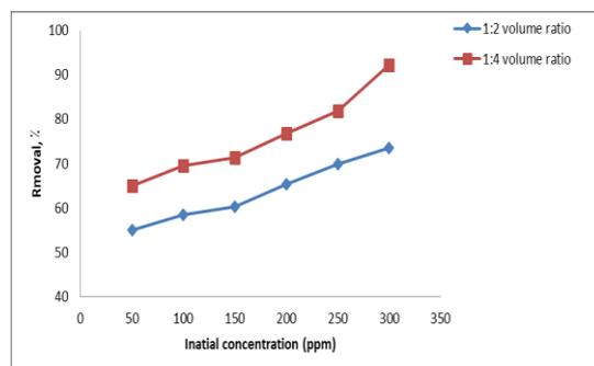
**Figure 14:**The relationship between initial phenol concentration and removal percent at (1:2, 1:4) volume ratio
