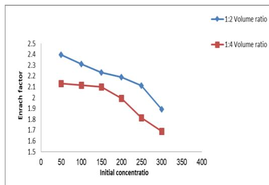
**Figure 16: The relationship between initial concentration and enrich factor for phenol at (1:2, 1:4) volume ratio**
