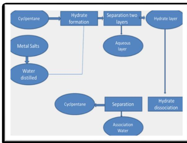
**Figure 2: Flow chart for experiments that separate pollutants from wastewater**
