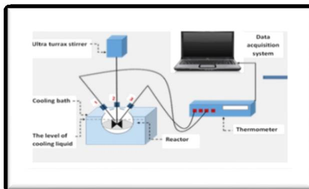
Figure 3: Hydrate formation cell for removal phenol
