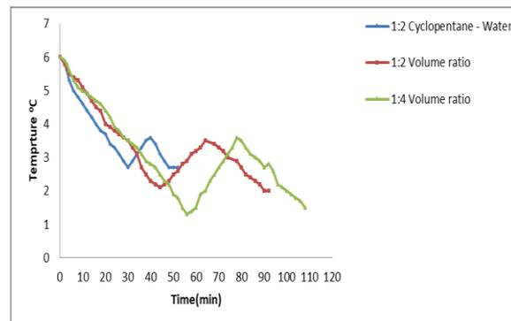
Figure 11: The formation rate CP Clathrate with phenol at 150 ppm and volume ratio 1:2 and 1:4
