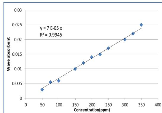
**Figure 5: Phenol standardization at various concentrations by Ultraviolet-visible Spectrophotometry**
