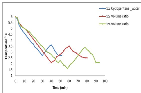
Figure 8: Formation rate CP Clathrate with phenol at 300 ppm and volume ratio 1:2 and 1:4
