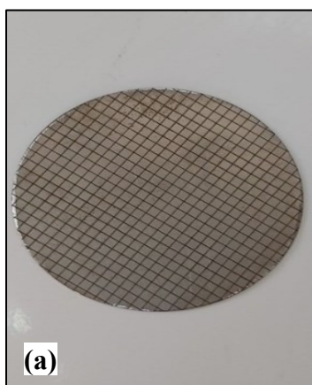
Figure 7: Drawing equipment; (a) blank used, (b) die set with a hydraulic press, and (c) the whole setup
