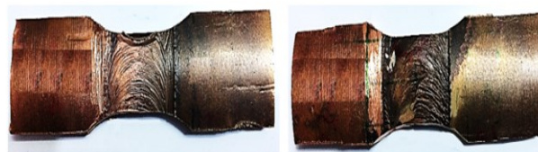
Figure 13: Sectioned of tension test specimens
