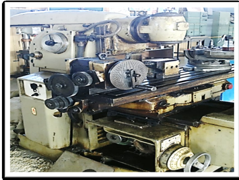
Figure 3: Conventional universal milling machine used in FSW
