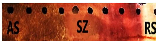
Figure 10: The distribution points of data for microhardness test of friction stir welding
