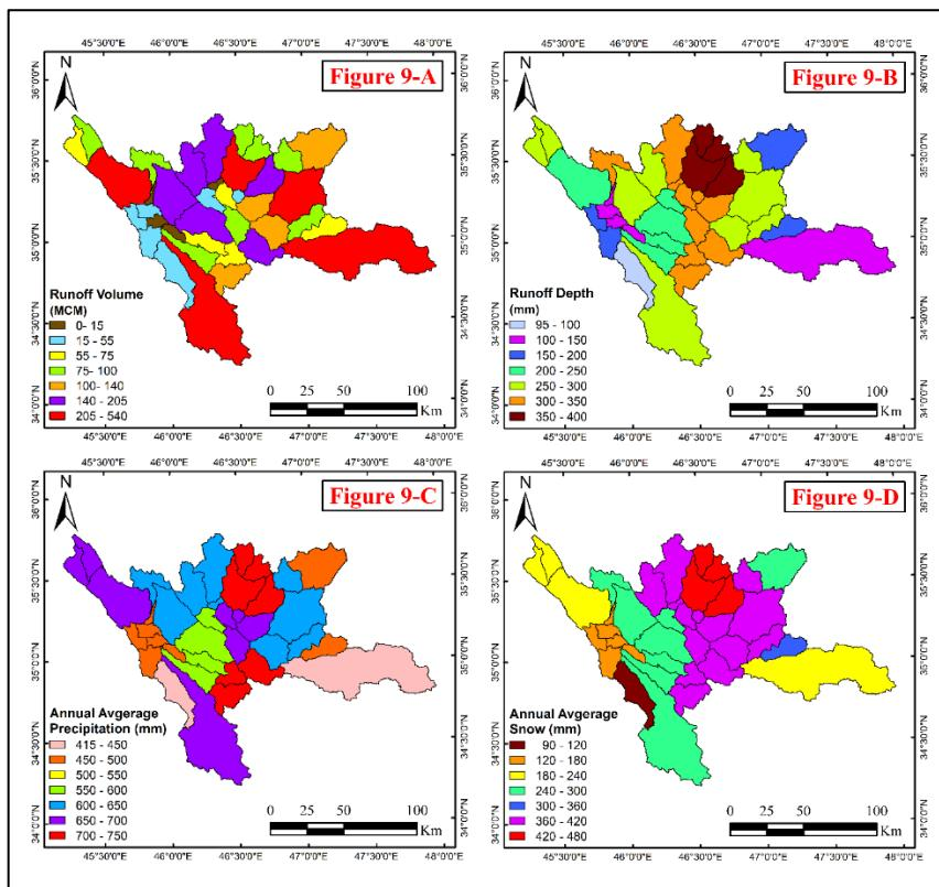
**Figure 9: Average spatially distribution from 1981 to 2008: A- Annual runoff volume, B- Annual runoff depth, C- Precipitation, and D- Snow**
