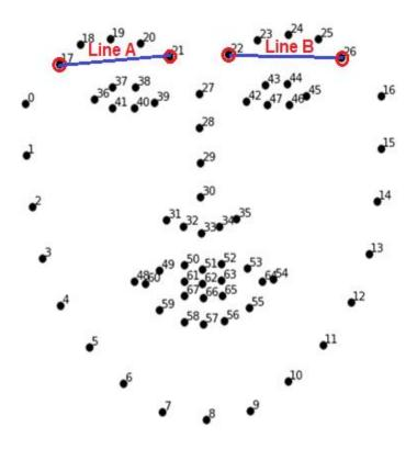
Figure2. Selected points for Yaw angle Calculation.
