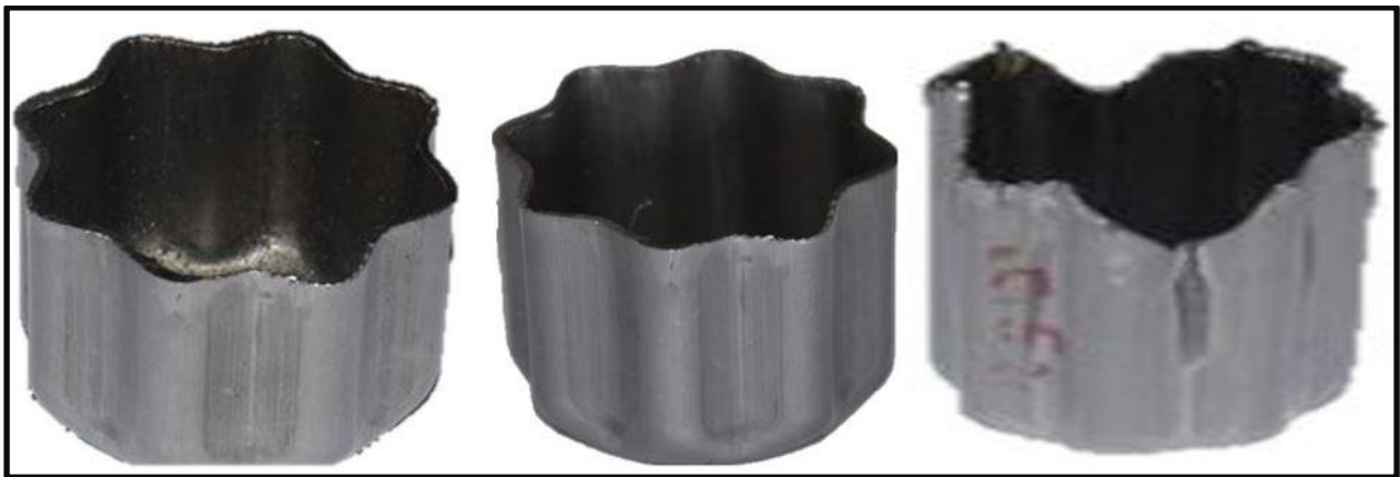
Figure 8: The astral cup produced with different radial clearance
