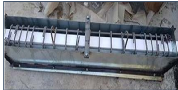
Figure 2: Mold with steel reinforcement and cork
