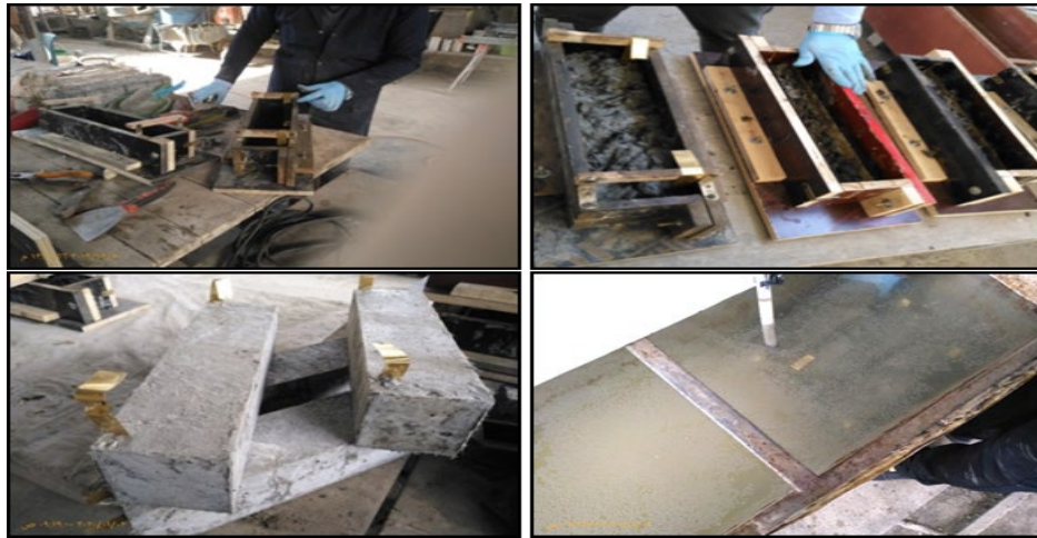
Figure 3: Preparation of smart cementitious composites sensors
