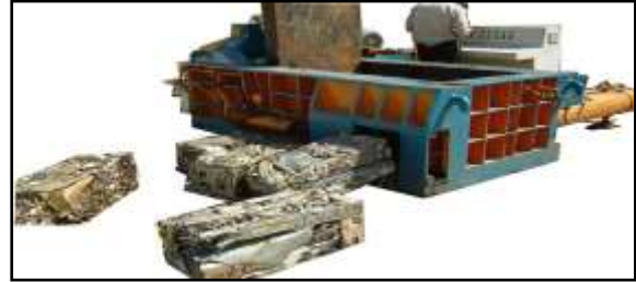
Figure 7: A type of hydraulic machine for producing bales [15]
