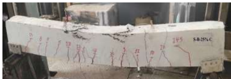
e) Failure mode of S-B 25% C beam.
