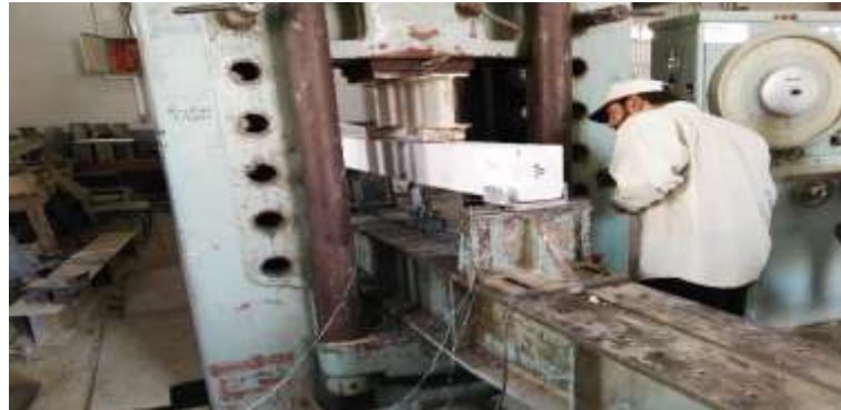
Figure 6: Testing of beam.
