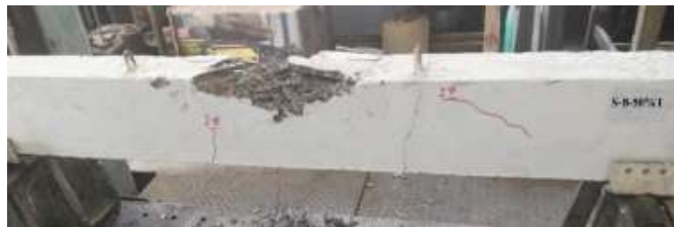
d) Failure mode of S-B 50% T beam.
