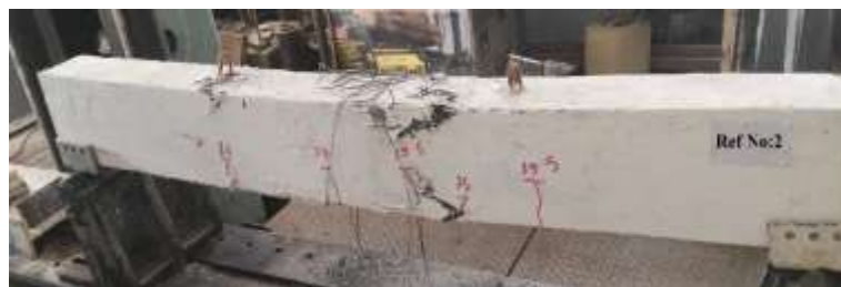
b) Failure mode of Ref No: 2 beam.
