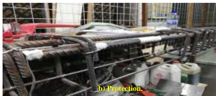
Figure 7: Strain gauge installation.
