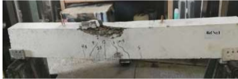
a) Failure mode of Ref No: 1 beam.
