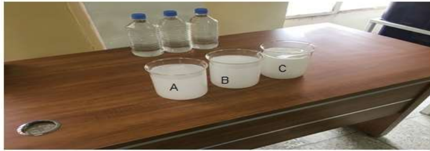
Figure 6: Nano fluid SiO 2 -H 2 O vol.conc. A- 0.1%, B- 0.2% and C-0.3%
