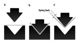
Figure 9: Illustration the springback in V- die.
