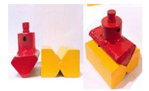
Figure 5: Shape of Die and Punch
