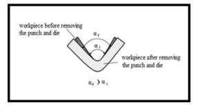
Figure 11: Illustrate the difference between final bending angle (af) and loading bending angle (ai)
