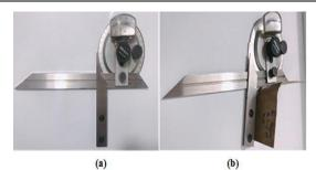
Figure 10: (a) Measuring device Mitutoyo 187-907 (b) the device while measuring the angle of the sample
