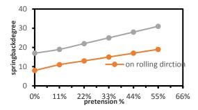
Figure 13: Variation of the measured spring back with pretension in two Directions
