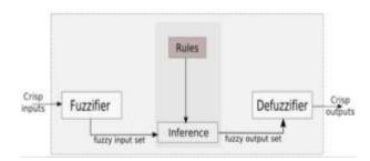
Figure 2: fuzzy logic controller system
