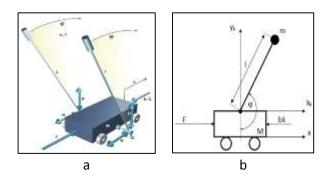
Figure 1: Inverted Pendulum cart, (a) 3-D view, (b) Side view
