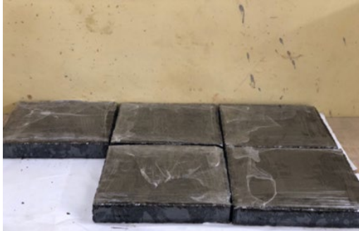
Figure 1: Slab models covered with Polyethylene
