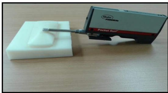
Figure 13: surface roughness measurement of a remote control shaped model
