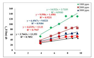
Figure 9: Pseudo-second -order kinetic model plot for different adsorbent dosage addition on biosorption of crude oil at pH 6.18, initial crude oil concentration 257.06 ppm, 250 rpm and 25 °C.
