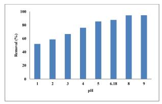
Figure 5: Effect of pH on removal percentage of crude oil at adsorbent dosage 5000 ppm, initial crude oil concentrations 257.06 ppm, 250 rpm, 25 °C and contact time 45 minutes
