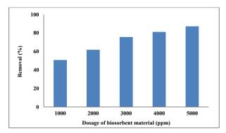
Figure 4: Effect of adsorbent dosage on removal percentage of crude oil at different adsorbent dosage, pH 6.18,250 rpm, 25 °C, initial crude oil concentration 257.06 ppm and contact time 90 minutes
