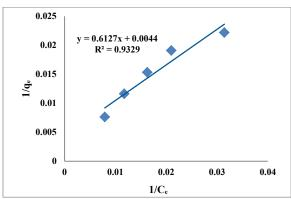
Figure 7: Linearized Langmuir isotherm model plot for biosorption of crude oil at pH 6.18, initial crude oil concentration 257.06 ppm, 250 rpm and 25 °C
