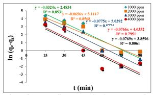
Figure 8: Pseudo-first-order kinetic model plot for different adsorbent dosage addition on biosorption of crude oil at pH 6.18, initial crude oil concentration 257.06 ppm, 250 rpm and 25 °C.
