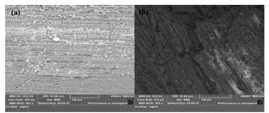
Figure 2: Scanning Electron Microscopy (SEM) analysis of papyrus reeds (a) before and (b) after crude oil adsorption
