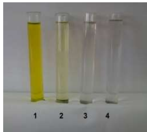
Figure 3: Physical separation between the aluminum chloride solution and silica by four times washing process with water.
