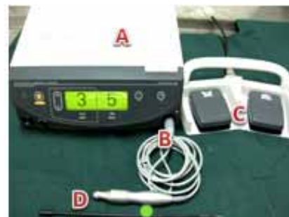
Fig.1: Ultrasonic device: Generator (A), Hand piece (B), Foot switches (C), Ultrasonic blade (D).
