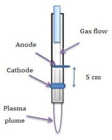
Figure (2) diagram of a plasma needle 1881
