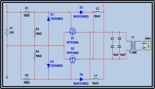
Figure 3. Electrical circuit of ZVS with flyback
