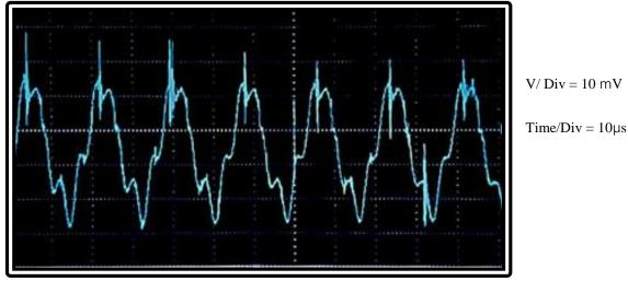
**Figure** 7. Output waveforms at the 47  $\Omega$  resistors
