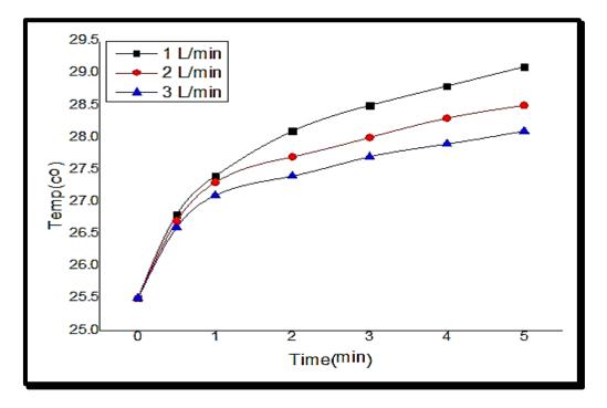
Figure 10. is the behavior of plasma temperature with time and for three gas flow states
