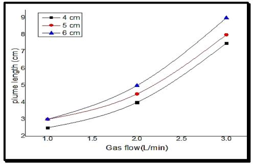
**Figure** 9. the behavior of the length of the plasma plume as the gas flow changes for three different distances between the poles (4,5,6) cm.
