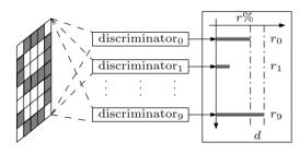
Fig. 2. Example of a weightless neural network consists of number of discriminators [16].
