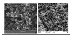
Figure 2: (a) Nano Al<sub>2</sub>O<sub>3</sub> with (10 - 20) nm and (b) Nano graphite powder with (20 - 40) nm
