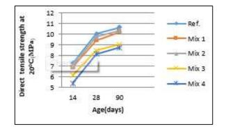
Figure 5: Direct tensile strength of RPC and RRPC at 20°C
