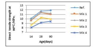
Figure 6: Direct tensile strength of RPC and RRPC at 90°
