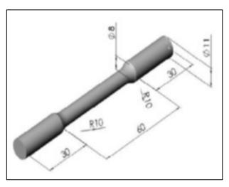
Figure 4: Tensile specimen's dimensions according to (ASTM E82) (All dimension are in mm)
