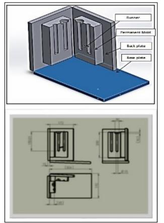
Figure 3: Sketch of mold with Dimensions (All dimensions are in mm)
