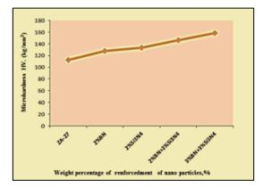
Figure 5: Micro hardness values of ZA-27 alloy and its composites
