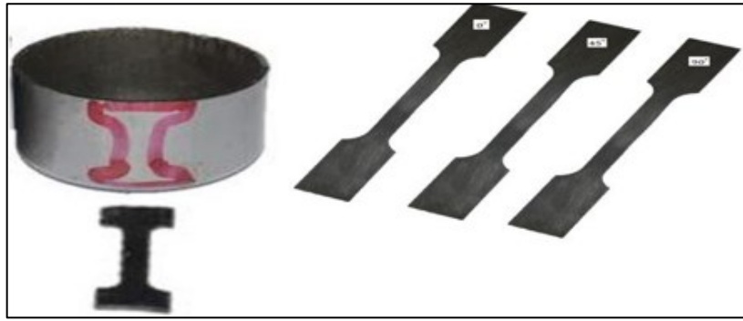
Figure 3: The specimens of unshaped blank and specimens were taken from a cylindrical cup
