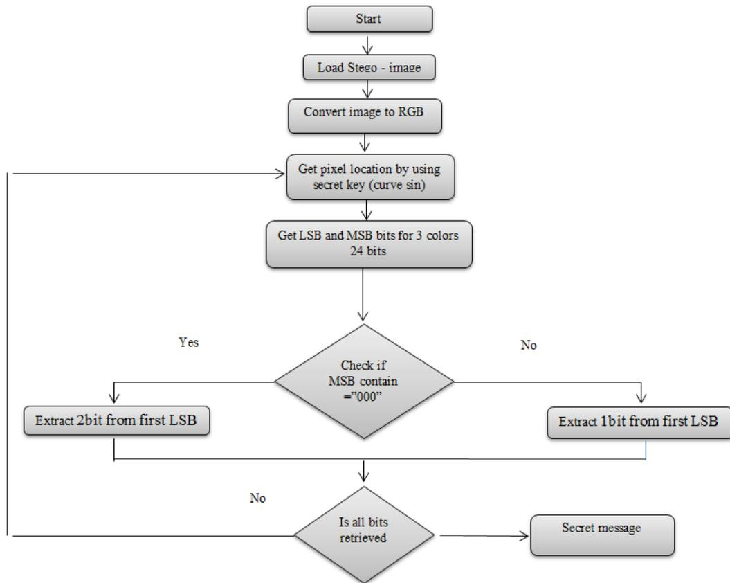
Figure 5: Flowchart extracting for receiving part.
