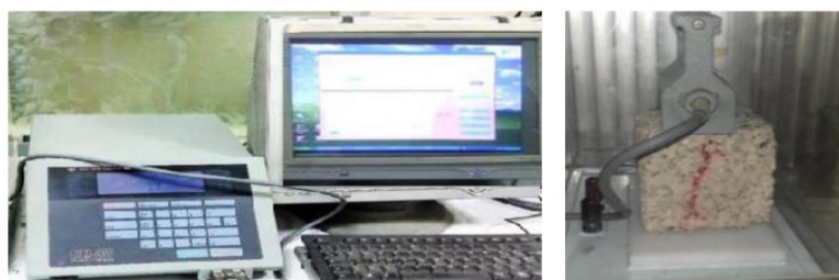
Figure 1: Device of PGC thermal conductivity test
