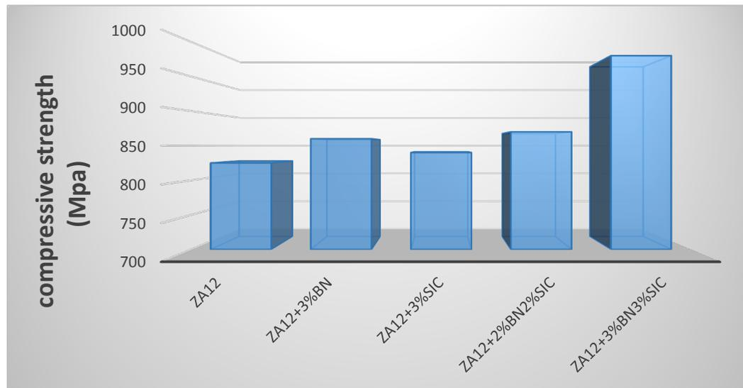
Figure 6: Compression values of ZA-12 alloy and its composites
