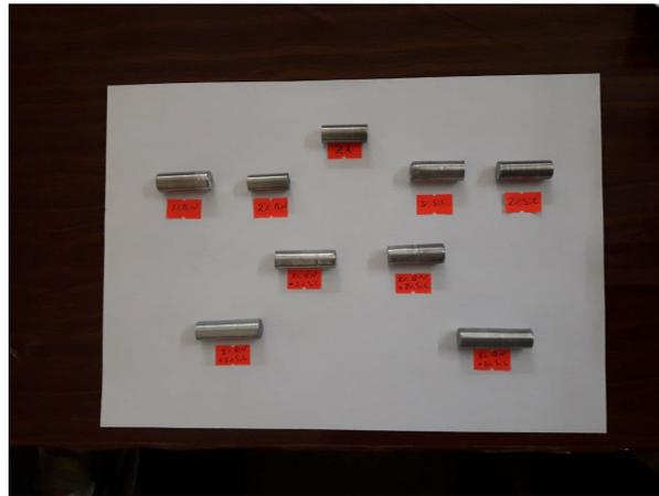
Figure 3: The ZA-12 alloy specimens with different weight percentage of nano particles reinforcement.
