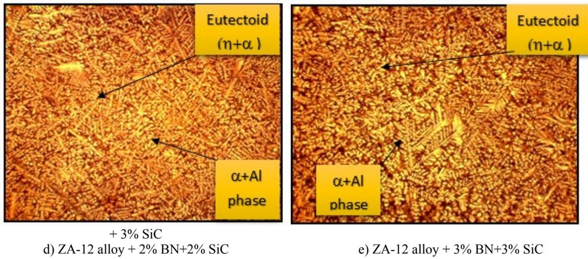
**Figure 9: The ZA-12 alloy microstructure of the matrix with the percent of nano particles at different weight and a magnification power of (10x).**
