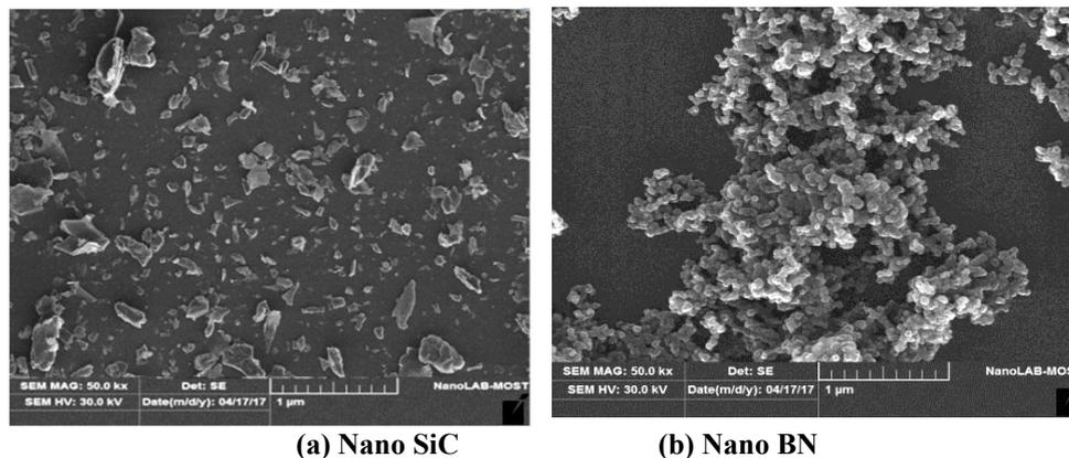
**Figure 1: (a) and (b) shows the SEM of the SiC and BN nano powders.**
