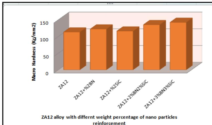
Figure 5: Hardness values of the ZA-12 alloy and its composites.
