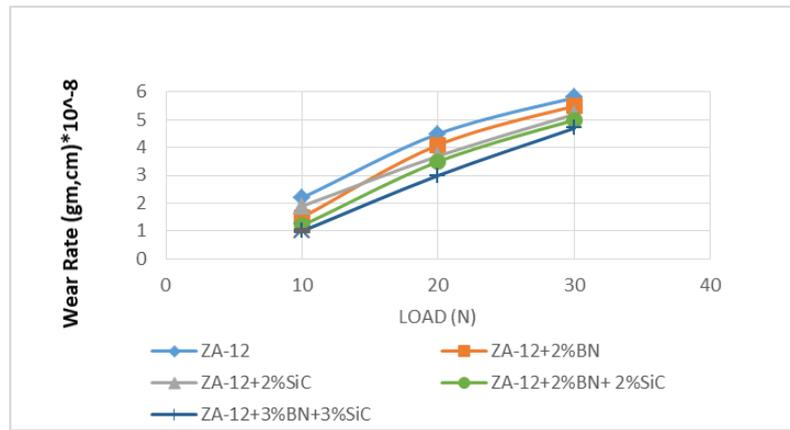
Figure 8: Wear rate values for ZA-12 alloy and its composites at different loads.
