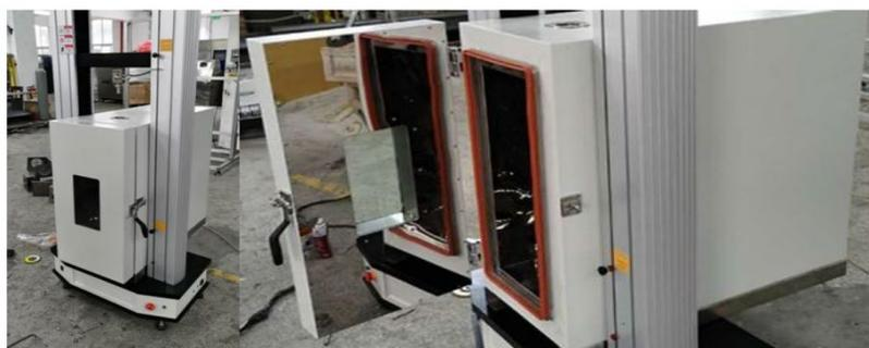
Figure 4: Final machine with the integrated oven
