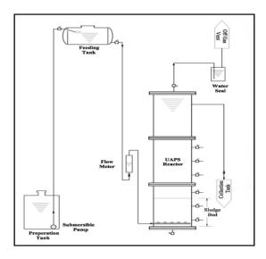
Figure 1: Schematic diagram of the UASB process.
