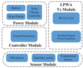
Figure. ( 3) main functional components of the monitoring node
