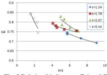
Fig. 3 Relationship between Fr1 and Cd for different values of expansion ratio
