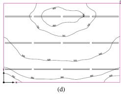
Fig 3. Luminous flux distributions: (a) incandescent lamp of 100W, (b) fluorescent with a conventional driver, (c) fluorescent with an electronic driver, and (d) LED-type luminaire
