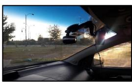
Fig. 2: Dash Camera Mounted in Windshield of Test Car
