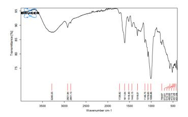
Figure (1): Pure cinnamon nanoparticle powder measurement by FTIR (Infra-red) spectroscopy
