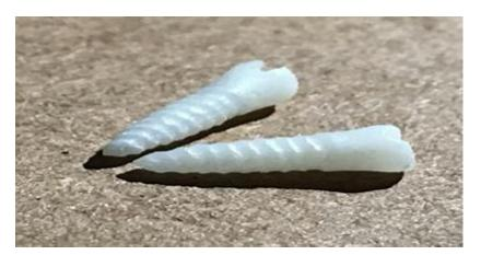
Figure (1): The digitally designed and manufactured zirconia dioxide implant.
