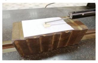
Figure (3): Specimen under stylus head during zirconia surface roughness measurement.
