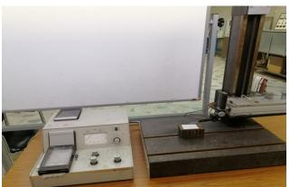
Figure (2): Profilometer device used in this study.
