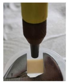
Figure (1): Specimen was fixed in a metallic tool for sandblasting procedure. Surface roughness evaluation
